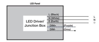
To wire multiple dimming panels to one standard 0-10v dimmer use the schematic below. The maximum number of panels that can be dimmed depends on the capability and capacity of the dimmer. Wire using plenum rated low voltage wire and appropriate connector. Each driver has a 2mA load on the control side, check the dimmer max control load. Aurora does not reccommed connection more than 20 panels together.
